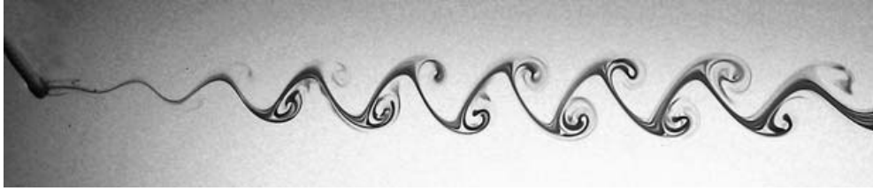
FIGURE 4. Kármán-Bénard vortex street behind a circular cylinder of diameter d = 0.478 cm moving with velocity U = 1.74 cm s -1 , Re = 83 .
